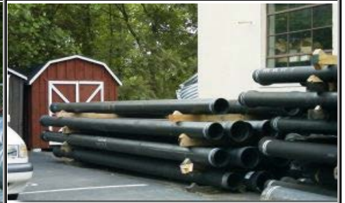
DIP, Ductile Iron Pipe – Water Main
